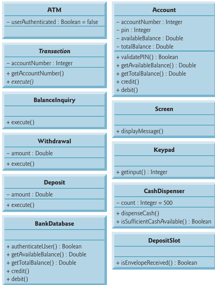
Fig. 13.10 | Class diagram with attributes and operations (incorporating inheritance). The abstract class name Transaction and the abstract method name execute in class Transaction appear in italics.
